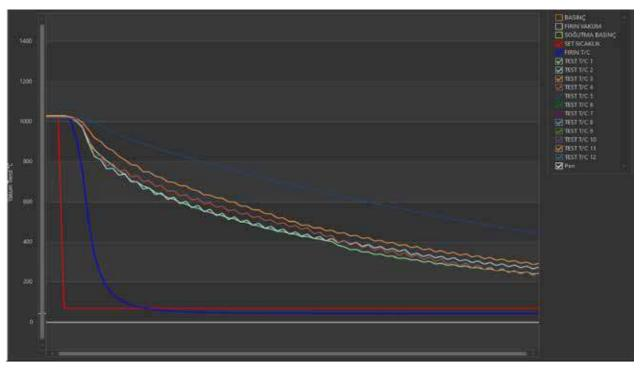
Figure 3. SCADA Temperature Trend Monitor During NADCA Test Cooling Phase
