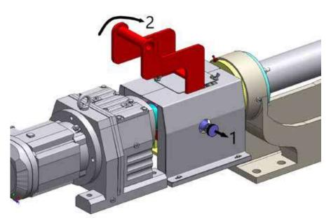
to be separated from the bed with the jack system, and maintenance was easily done. The role to be replaced was easily removed from a single cover in this way that we achieved our goal of minimizing maintenance times by ensuring that the beds are separated in a much shorter time than normal.
