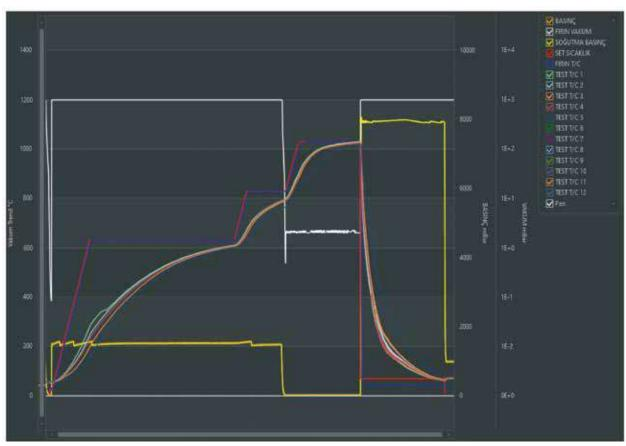
In Figure 3, it is observed that the surface thermocouple curves have a zigzag-like increasing and decreasing character due to the core temperature being higher than the surface temperature, depending on the direction changing time of the diverter caps that enable the nitrogen, which is the refrigerant gas, to be directed from
