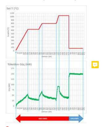
Figure 4. Energy Consumption Graphic of NADCA Test
